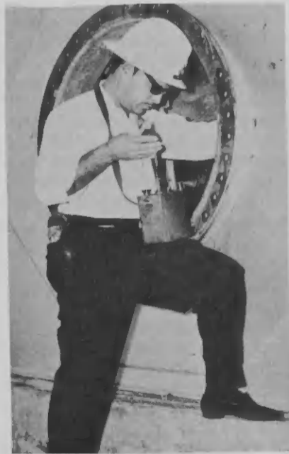
C. KROZENDIJK performs gas test in tank.
